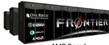
AMD Based (Up & running) 20 MW
